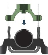
The K-Line tapping saddle should sit snugly over the tubing without a gap.
