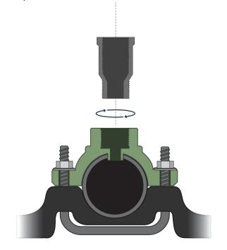
Hand start the impact sprinkler (careful not to cross thread), then finish tightening with a 20mm open ended wrench or channel lock pliers.
