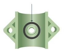
Push the K-Line tapping saddle down over the threaded posts and be certain that the nipple on the underside of the tapping saddle is inserted into the 14mm hole.
