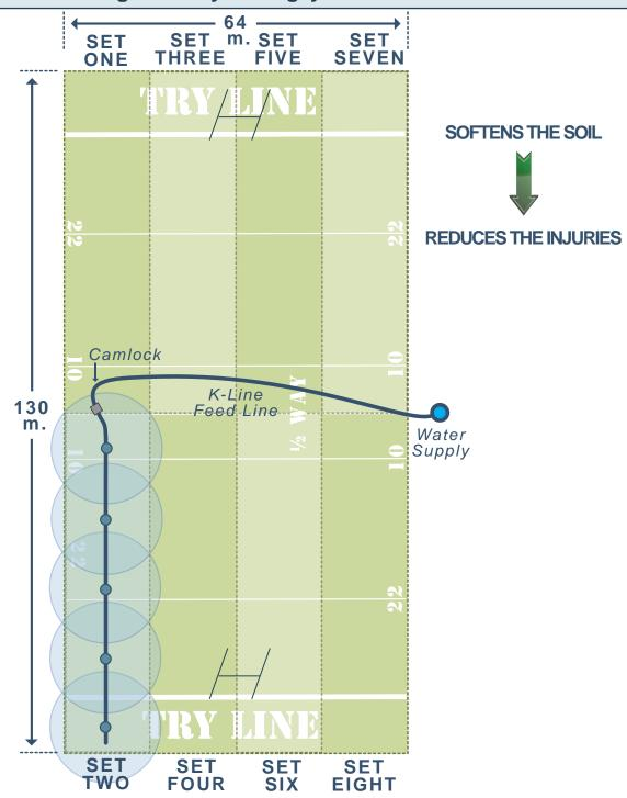
This design can be used for football or soccer fields and consists of a 5 pod system with 8 sets or shifts.
