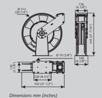
Full metal Intensive Duty double pedestal hose reels, with hose capacity up to 15 m x 1/2" hose.
