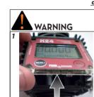
Carefully remove the screws from the corners of the front panel, and then carefully lift the front cover up way from the main body of the meter.
