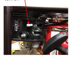
Fill engine with oil to correct level
