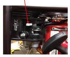
After use drain water from casing \
