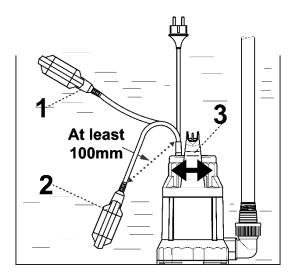
The pump will start pumping when the fluid has lifted the float switch fully (1).
